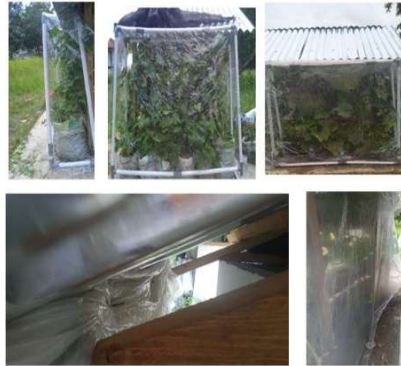
Figure 4. Modified in-chamber method to measure CO 2 concentration
