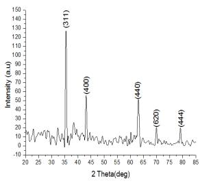
**Figure 1.** The XRD diffraction pattern of the MgFe<sub>2</sub>O<sub>4</sub> nanoparticle
