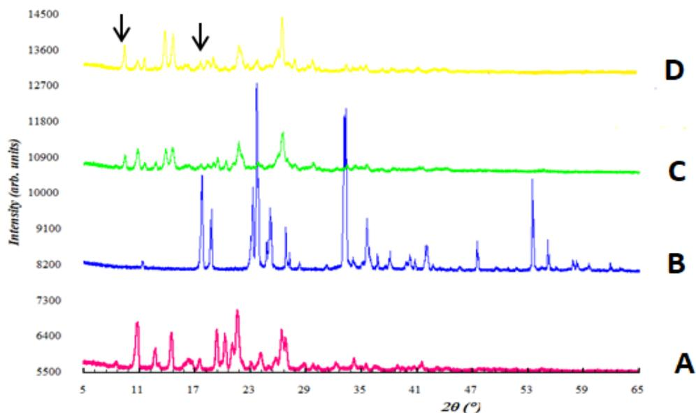
**Figure 1.** Powder X-ray diffractogram of (A) MLX, (B) MA, (C) PM, dan (D) *Slurry* cocrystal
