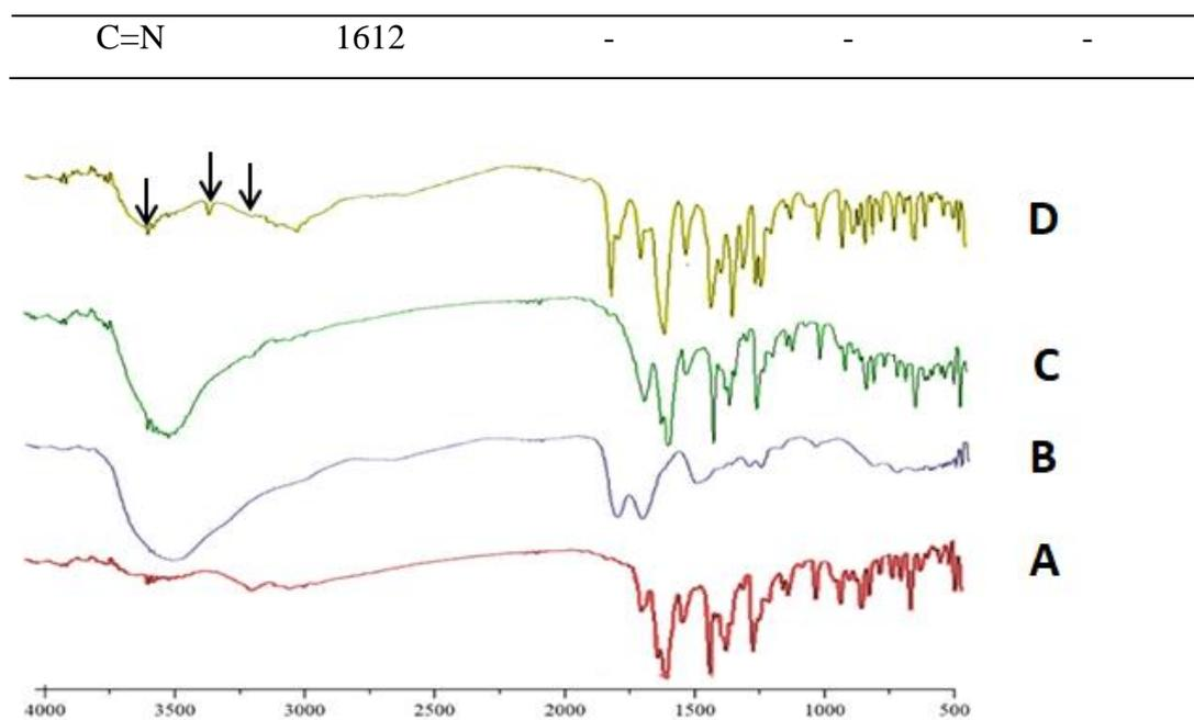
**Figure 3.** Infrared spectra of (A) MLX, (B) MA, (C) PM, and *Slurry* cocrystal
