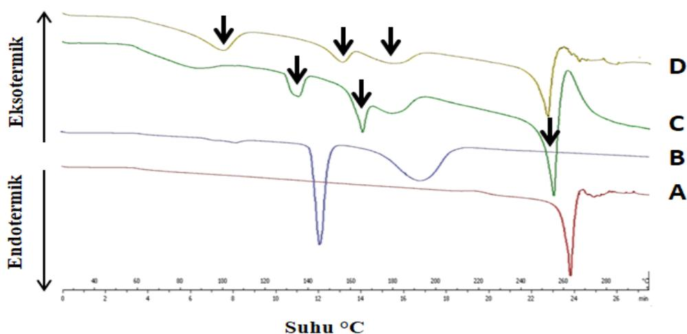
**Figure 2.** Thermogram of (A) MLX, (B) MA, (C) PM, and (D) *Slurry* cocrystal**Table 3.** Comparison wavenumber of MLX , ASM, CF, and *Slurry* cocrystal
