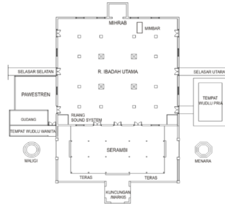
Figure 4. Building plan of Al-Wustho Mangkunegaran Mosque [3]
