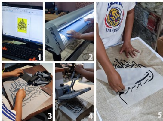
Figure 8. Step by step in processing digital screen printing
