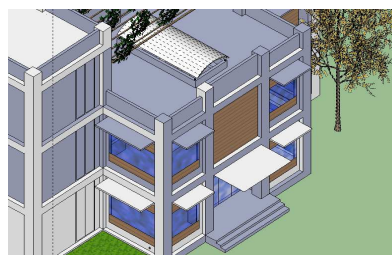
Figure 6. The addition of green canopy and roof insulation.( Source: Observation, 2012)
