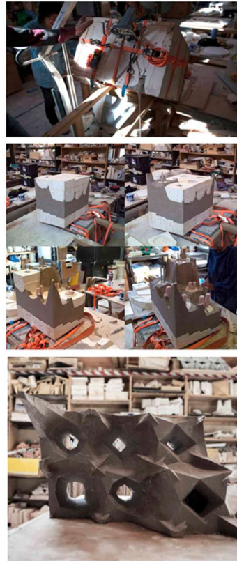
Figure 38. Steps involved in slip casting
