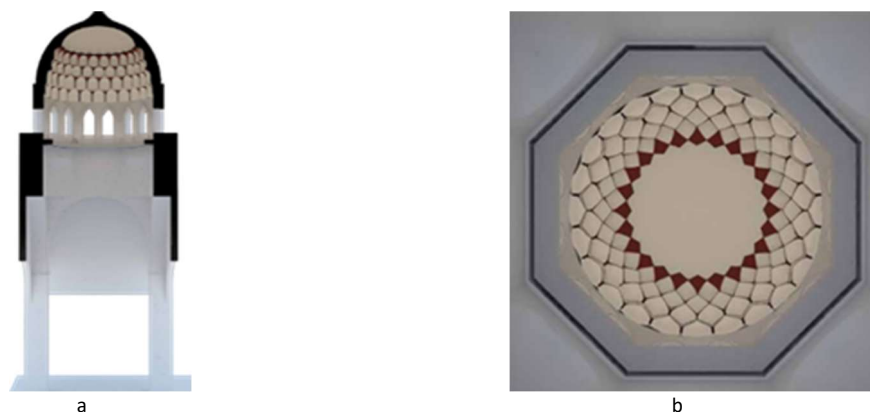
Figure 6. (a) Section of the Dome of the Eagle after applying the Ayyubid era muqarnas; (b) Applying the muqarnas of the citadel's eastern entrance inside the Dome of the Eagle
