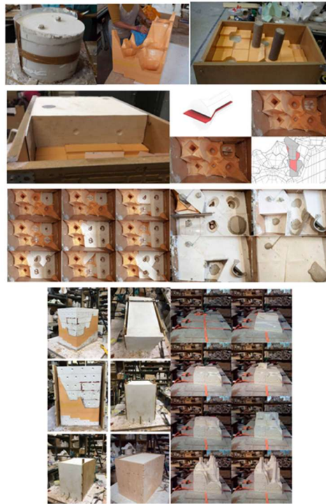
Figure 37. Steps of Fabrication of the Plaster Mold
