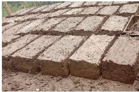
Figure 2. Sun-dried mud brick (known as labin )
