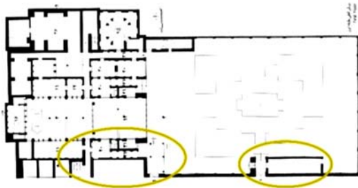
Figure 7. Ground floor of Angurestan malek. This building has two entrances with different features. The entrance that opens to garden cannot block the visual relation. But entrance that is next to the building uses some turnings to do this.[20]
