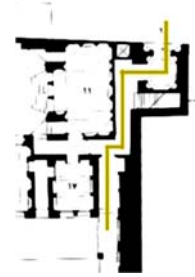
Figure 8. Parts of ground floor of Bakuchi house. In this plan, entrance is shown and a path indicates the movement flow in it. It shows how patterns of transition and pause work in entrances. [14]
