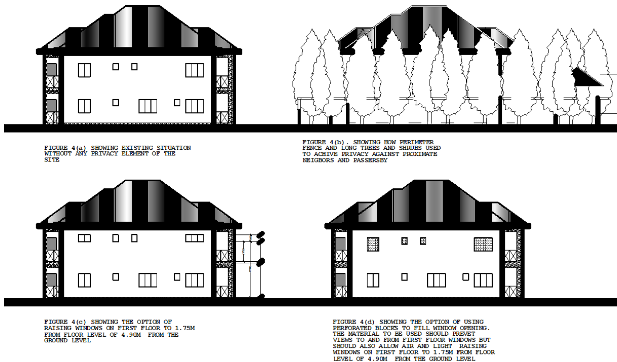
Figure 4 (a, b, c & d) Using western side elevation of the floor plan to show options for achieving privacy on the first floor against proximate neighbors and passersby. For example, the use of shrubs and trees (a), raised window level to 1.75m from suspended floor level or 4.90m from ground floor level (b) and ingenious use of perforated blocks or Aluminum foil to screen windows (e) (Redesign: Authors, 2017)
