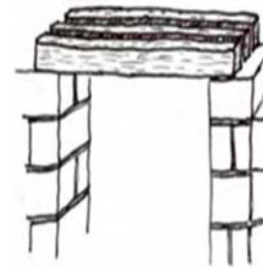
Figure 7. Timber thresholds to cover the holes, "Doors and Windows"
