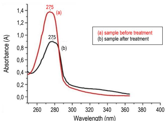
**Figure 4.** UV-VIS spectra of the sample before the electrocoagulation process and the sample after the electrocoagulation process
