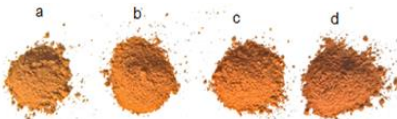
Figure 2. Goethite obtained at (a) 60°C (b) 70°C (c) 80°C (d) 90°C of synthesis temperature
