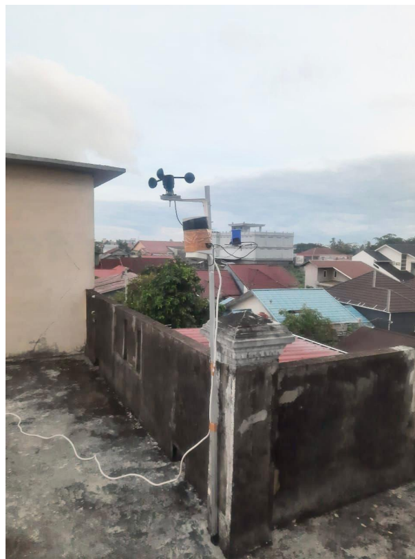
Fig. 1: The IoT-based weather monitoring system deployed in Pontianak City for high-frequency wind speed data collection
