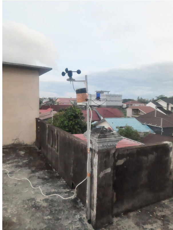
Figure 1: The IoT-based weather monitoring system deployed in Pontianak City for high-frequency wind speed data collection
