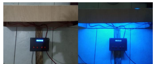
Figure 3. Phototherapy tools with temperature sensor and timer
