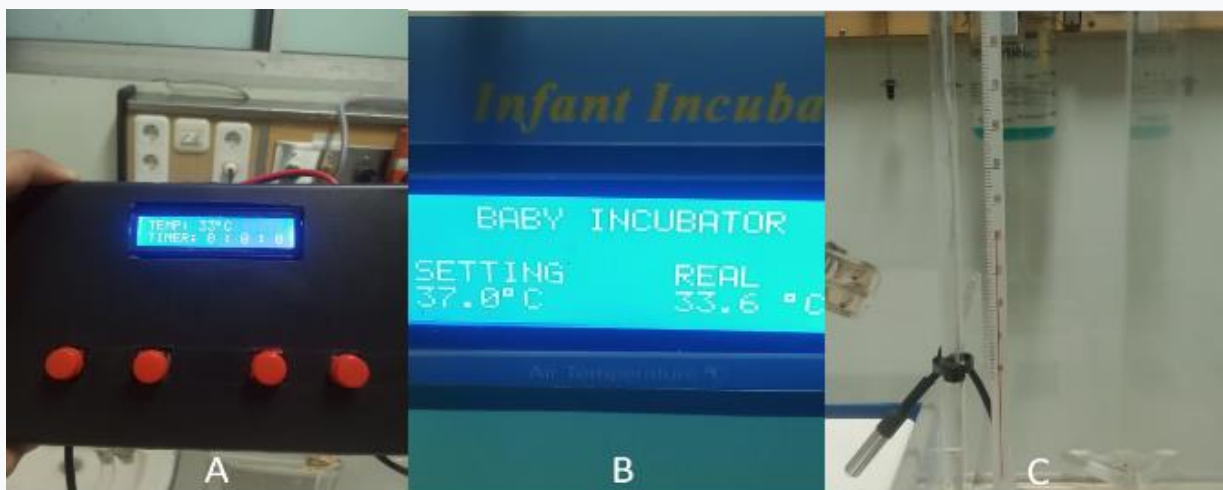
Figure 5. Testing temperature sensor. (A) Phototherapy tool (B) baby incubator in hospital (C) Thermometer
