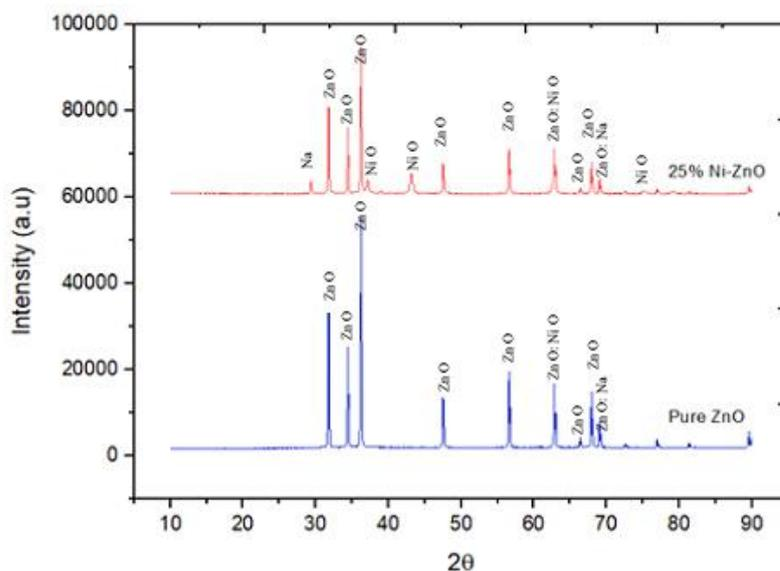
**Figure 9.** XRD pattern of pure ZnO and ZnO photocatalyst samples with 25% Ni addition concentration.
