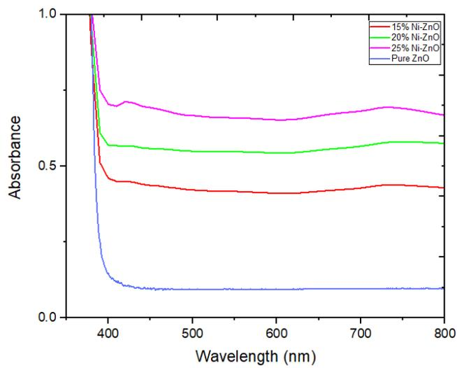
**Figure 5.** Optical absorption graph of the ZnO photocatalyst sample with variations in the addition of Ni 0, 15, 20, and 25%
