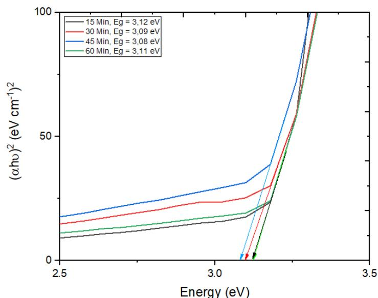
**Figure 8.** Graph of the band gap width of the ZnO photocatalyst sample with variations in sonication time of 15, 30, 45, and 60 minutes
