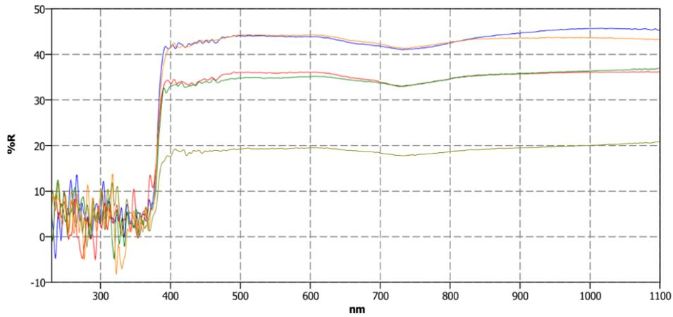
**Figure 4.** Ni-ZnO photocatalyst sample optical reflectance graph
