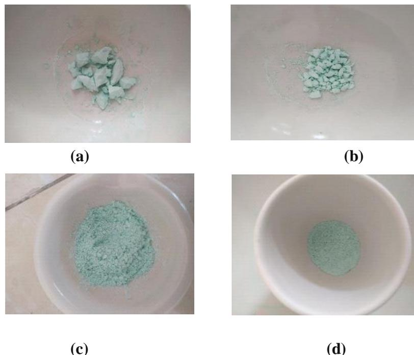
**Figure 3.** Sample (a) 15 minutes sonication (b) 60 minutes sonication after calcination (c) 45 minutes sonication (d) 60 minutes sonication after crushed
