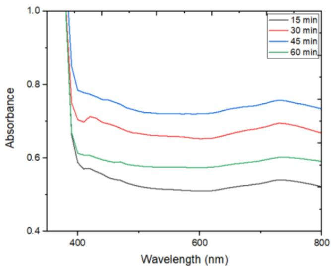
**Figure 6.** Optical absorption graph of ZnO photocatalyst samples with variations in sonication time of 15, 30, 45 and 60 minutes
