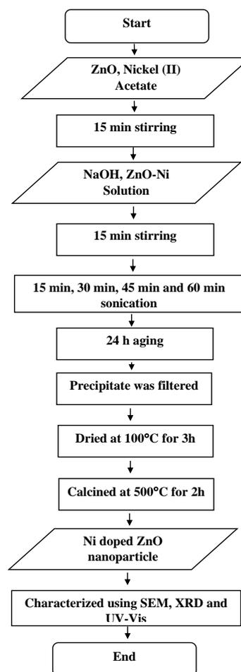
**Figure 1.** Flowchart of the synthesis of Ni-ZnO
