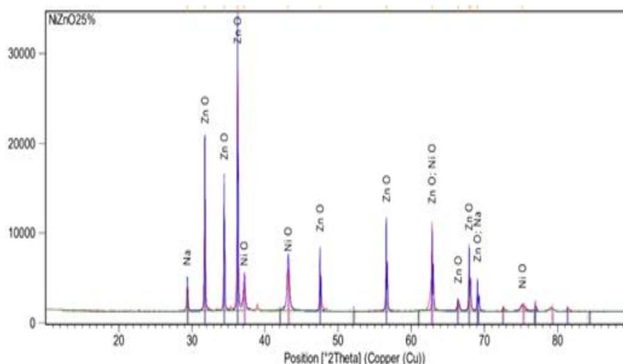
**Figure 10.** X-Ray Diffraction Peak Analysis of 25% Ni - ZnO sample
