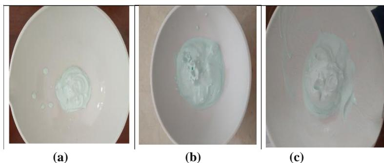
**Figure 2.** Sample (a) 15 minutes sonication (b) 45 minutes sonication (c) 60 minutes sonication.
