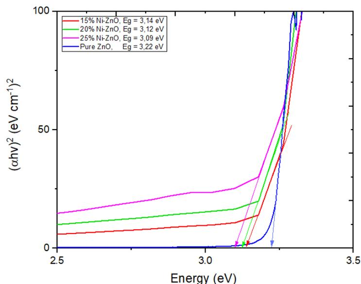
**Figure 7.** Graph of the width of the band gap of the ZnO photocatalyst sample with variations in the addition of Ni 0, 15, 20, and 25%
