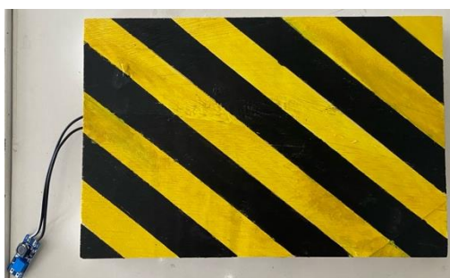
Figure 10. Prototype of a CDs-doped Zn layered piezoelectric sensor as a speed bump
