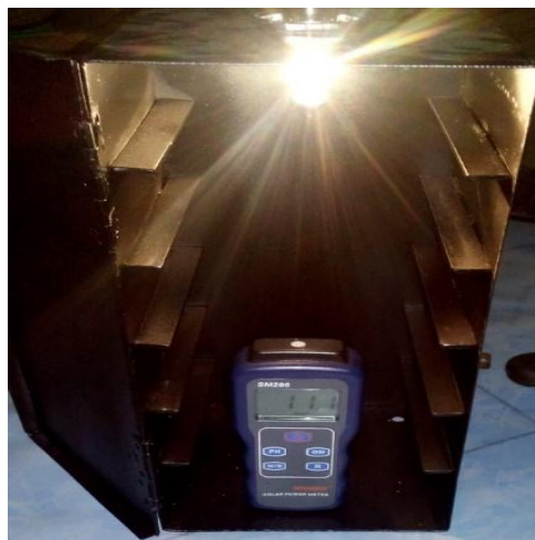
Figure 1. Sun simulator using hologen bulb lamp.
