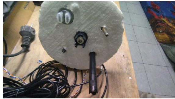
Fig 16. Placement of sensors on styrofoam buoys
