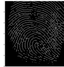
Figure 12. Fingerprint image of Zhang-Suen's thinning processing
